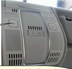
Open the car door to turn courtesy light on, or press the button to start transmitting a code to open the gate, garage door or barrier.
