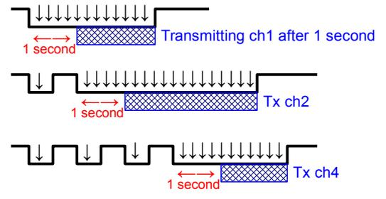
**Sender in pulsed mode** (1÷4 channels transmitter/duplicator): starts transmitting after 1 second from switch being pushed: 1 pulse=>ch1; 2 pulses=>ch2; 3 pulses=>ch3; 4 pulses=>ch4
