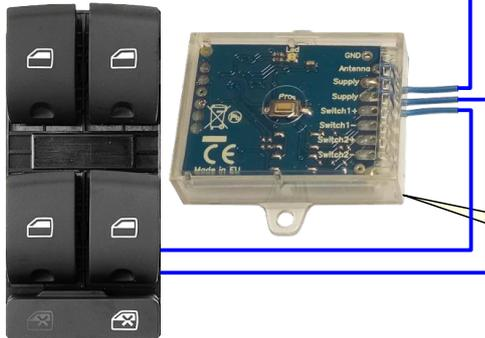
Power supply range in pulsed or car mode: from 12 to 27Vac or from 12 to 36Vdc
