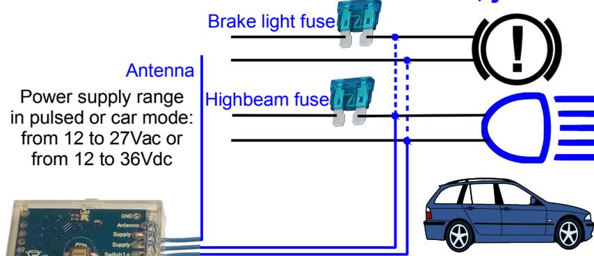
Power supply range in pulsed or car mode: from 12 to 27Vac or from 12 to 36Vdc
