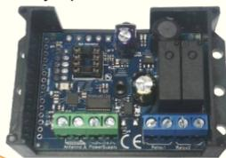
**Door opens => NC will be shorted to COM so SenderBatt starts transmitting code #1 => UniRec2 opens Relay1 output => safety OFF => garage door cannot be opened (motor disabled).**
