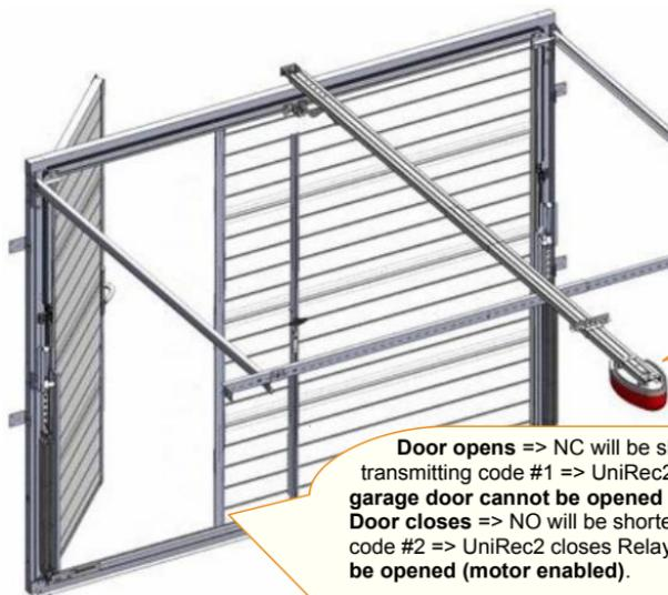
Relay1 configured in bistable ON/OFF, and connected to the motor operator safety input.
