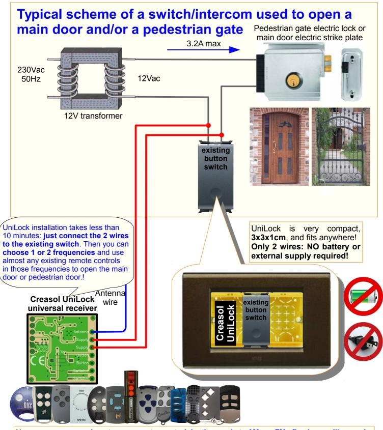
Now you can use almost any remote control in the market, AM or FM, fixed or rolling code, to open your main door, pedestrian gate or any other system using an electric lock.
