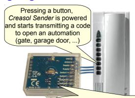
Sender in basic mode (1 channel transmitter/duplicator):
